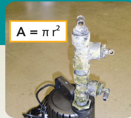
One 1 1/2" pipe = Nine 1/2" pipes
