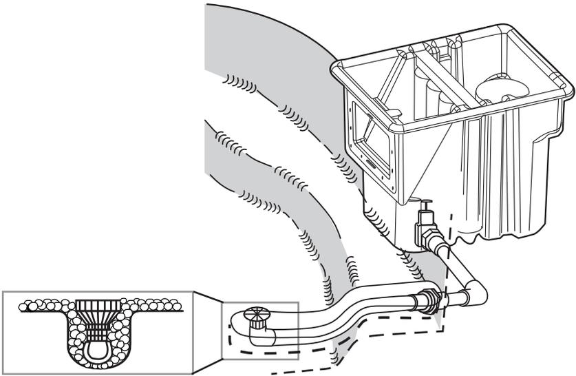
Drill-points have been provided on all compatible Skimmer models to show the proper location for the bulkhead fitting. See Figure 17. Drill the hole with a 3" hole saw and install the bulkhead following the bulkhead installation instructions on page 9.
