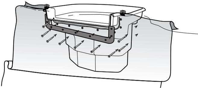
Attach the liner flange to the FilterFalls, starting with the center screw first, and then work out toward the sides of the spillway. It may be necessary to first pierce the liner with a nail or an awl before inserting the screw. Do not fully tighten any screws until all the screws have been installed. Once completed, trim away any excess liner as needed.
