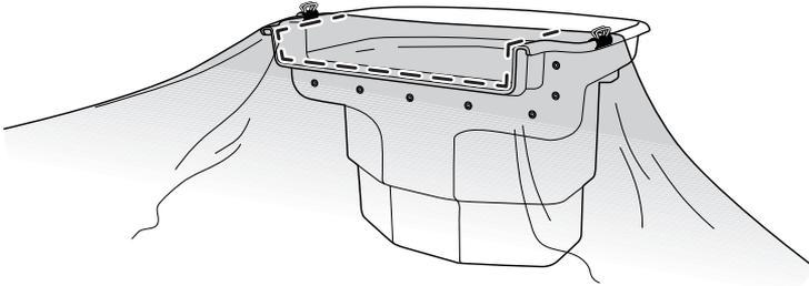
Remove the spring clips and pull the liner away from the face of the enclosure. Make sure that the front of the FilterFalls and the back side of the liner are clean and free of debris. Apply a consistent bead of Atlantic fish-safe silicone to the face of the FilterFalls along the center line of the threaded inserts.
