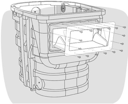
Use your fingers to hold the flange nut and a hand held screwdriver to tighten the screws. The serrations on the flange nut will grab the plastic enclosure once it makes contact, eliminating the need to use a wrench. Use caution when tightening the screws. The screws need only be snug for the silicone to make a seal.
