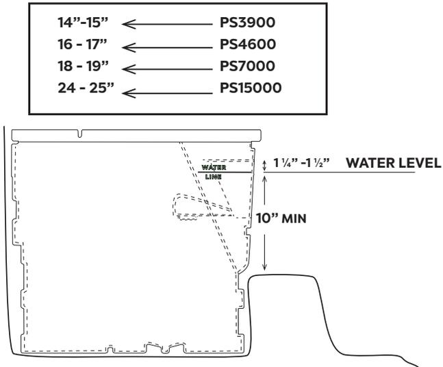
Place the Skimmer enclosure into the excavated hole. Check the top of the enclosure to make sure that it is level front-to-back and side-to-side. Check where your pre-determined water level falls on the face of the Skimmer enclosure. The water level needs to be between 1/4" and 1 1/2" below the top of the weir door opening and even with the water level indicator molded on the side of the Skimmer. (PS15000 only)
