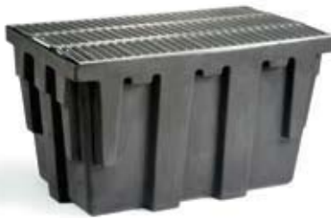
Model: SEC250 Dimensions: 46"W x 29"D x 27"H Max Pump Flow: 10,000 gph Capacity: 100 gal Grate: Galvanized steel
