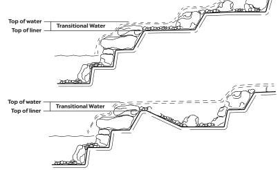
Below is an example of improper streambed construction. Stone, gravel and foam can be combined to make a barrier and create a waterfall, but that barrier will never be watertight. When the pump is turned off, the water will always drain down to the highest point of the liner. Improper construction greatly increases the water in transition.
