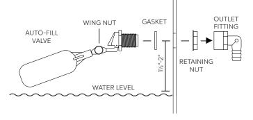
The Auto Fill Kit includes fittings for connection to a garden hose,  $\frac{1}{2}$ " irrigation line, and  $\frac{1}{2}$ " Sch 40 PVC. Wrap the  $\frac{1}{2}$ " male threads on the Auto Fill with thread sealant and install the fitting of your choice. Once water is supplied to the Auto Fill it will maintain the set water level by automatically adding water when the level drops. This level can be adjusted by loosening the wing nut and raising and lowering the height of the Auto Fill float.
