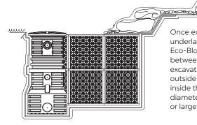
Once excavation is complete, install underlayment, pond liner, properly oriented Eco-Blox and Pump Vault. Backfill the space between the Eco-Blox/ Pump Vault and the excavation to lock them into place, either outside the liner with sand or clean fill, or inside the liner with gravel ¾" or larger in diameter. Top the liner and basin with ¾" or larger gravel or decorative stone.
