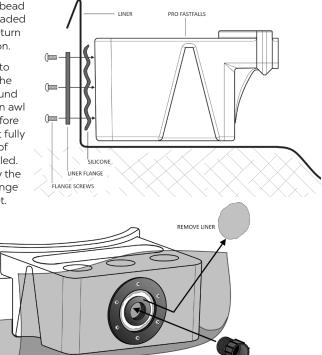
Tighten flange screws with a hand held screwdriver only. Over tightening the screws could strip out the inserts or crack the liner flange. The screws need only to be snug for the silicone to make a seal.
