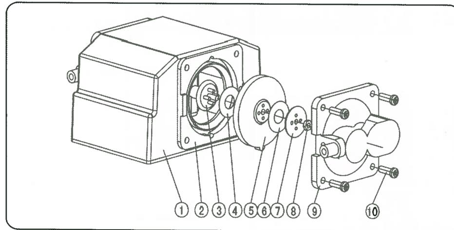
The most common cause of premature diaphragm failure is excessive back pressure or overheating. This can be caused if the pump is producing too much air for your diffusers, or if the tank is too deep for your pump. The depth of the tank should be as follows:
