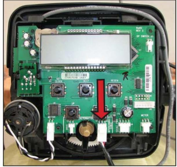
5. Connect each end of the 8' alternator interconnect cable to the three pin connector labeled **INTERCONNECT CABLE**, on both Control Valve Alt. "A" and Control Valve Alt. "B".
