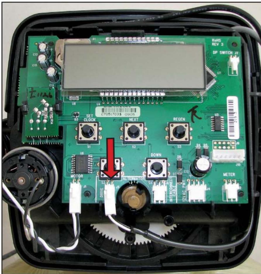
4. The 8' alternator valve motor cable must be connected to the two pin connector labeled **DRIVE** on Control Valve Alt. "A".
