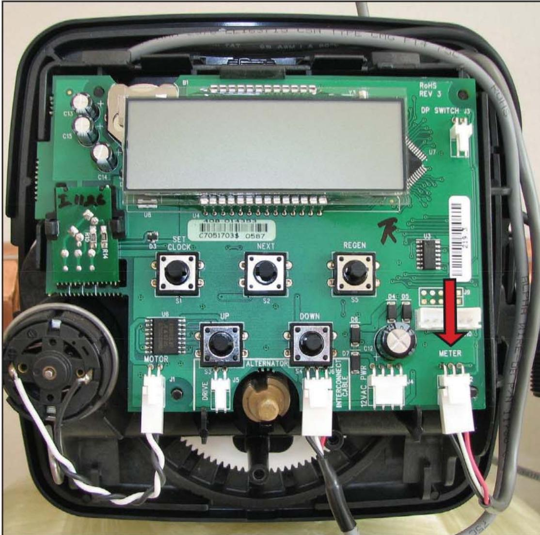
6. **SINGLE METER APPLICATIONS:** Connect the 15' water meter cable to the three pin connector labeled **METER** on either Control Valve Alt. "A", or Control Valve Alt. "B". **NOTE: Due to the number of wires coming through the back plate, this connection can be made more easily on Control Valve Alt. "B".**
