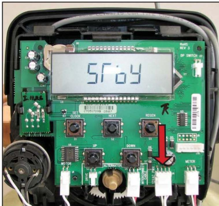
7. Connect the power cable to both of the four pin connectors labeled **12VAC PWR** on Control Valve Alt. "A" and Control Valve Alt. "B". The control valve will now be ready for programming.
