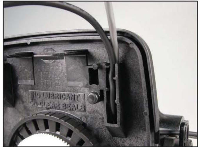
3. Route the wires through the back plate and weave them through the retainer. Allow about one foot of cable through the back plate to allow for connection to PC Board.
