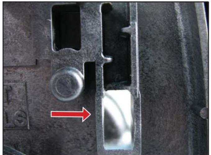
2. With needle nose pliers break off the plastic tabs on each side of the back plate. When tabs are removed you are now able to run two wires through each side of the back plate.
