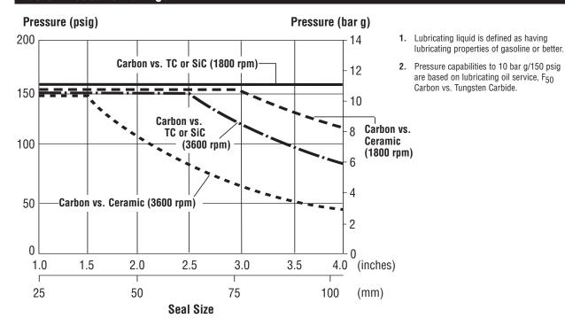
The Basic Pressure Rating is for a standard Type 21 seal, as shown in the typical arrangement, when installed according to the criteria given in this data sheet and generally accepted industrial practices.
