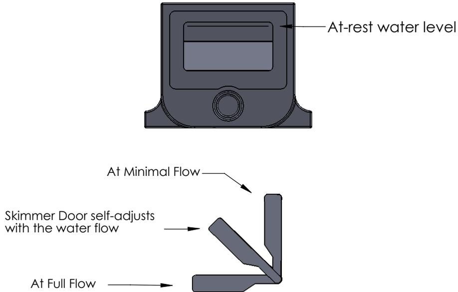
The highest water level in the pond matches the in-tank overflow level.
