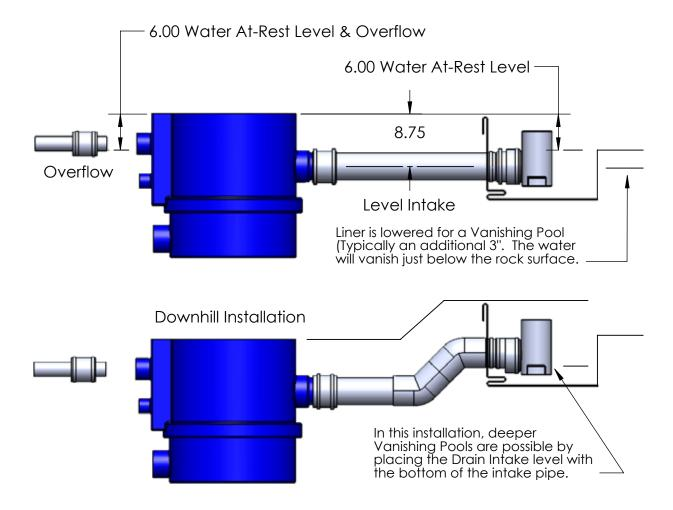
The At-Rest water level in the pond is determined by the overflow level inside the Filter Tank. The highest overflow level is 2.50" down from the top of Filter Tank.
