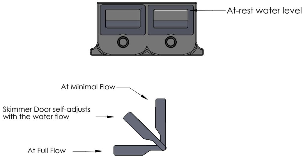
The highest water level in the pond matches the in-tank overflow level.
