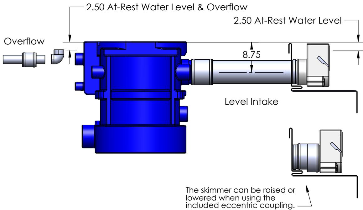
The At-Rest water level in the pond is determined by the overflow level inside the Filter Tank. The highest overflow level is 2.50" down from the top of Filter Tank.
