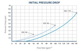
Pressure drop shown above is for filter housing and 20 micron filter cartridge in clean water.
