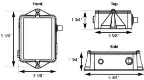
TimerMicrocontroller with triac outputTurndown Ratio10:1HousingPolycarbonate plasticShipping Weight2 lbs (1 kg)
