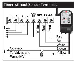
4. Attach the Red wires to the timer's 24 VAC power terminals.
