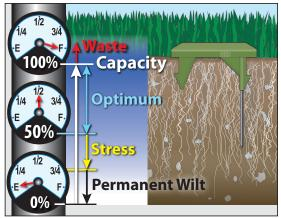
adjust the setting incrementally from 0% to 100%, the Precision system can be fine-tuned for virtually any soil condition.
